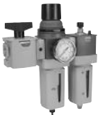
Ball Valve + Filter/Regulator + Lubricator Combinations, poly bowl 5 micron element, 116 psig (8 bar) regulator + gauge and wall mounting brackets
